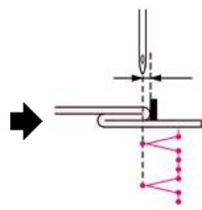
Turn the handwheel to check the needle entry point.
