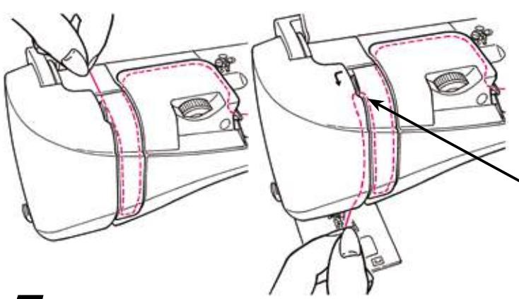
\* Check that the thread take-up is correctly threaded.
