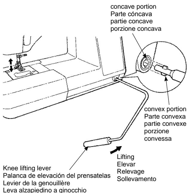
The knee lifting lever is useful when a quilt is being sewn and for other projects that require the use of both hands. With the knee lifting lever, you are able to control the position of the presser foot without using your hands.
