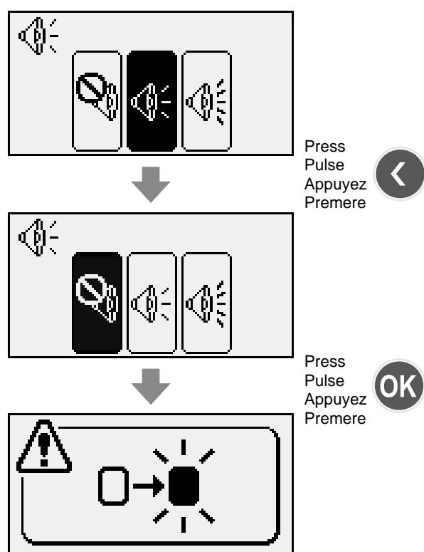
**Now the volume setting is changed and it will not produce a sound even when a button is pressed.**
