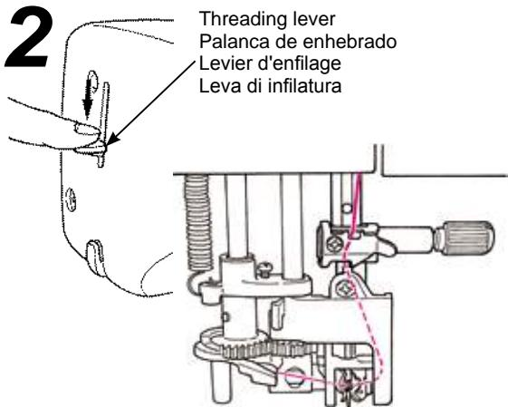
● Lower the threading lever until it comes to a complete stop.
