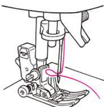
● Release the threading lever and the needle thread is threaded to the needle eye.
