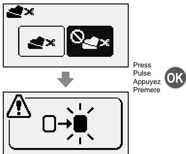
**The thread trimming foot switch is now turned off.**
