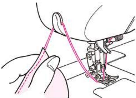
\* You can also cut the threads by the thread cutter at the face plate cover.
