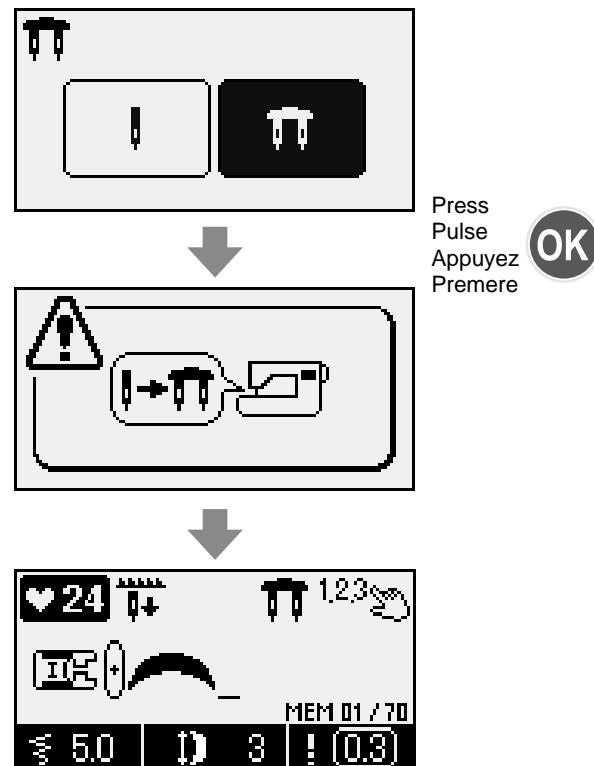
**Symbol of twin needle sewing will be shown on the display.**
