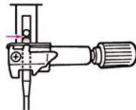
It is impossible to perform stitching if the needle is not correctly installed or a bent needle is used. Pay close attention as this will cause machine malfunction.
