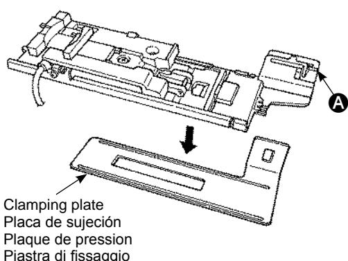
It will be easier to sew buttonholes on the thin fabrics and/or near the overlapped sections, if the clamping plate is used.
