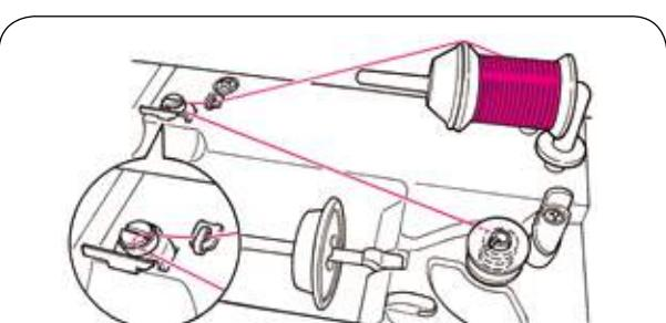
\* Bobbin winding is also possible with supplementary spool pin.
