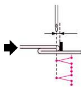
Turn the handwheel to check the needle entry point.
