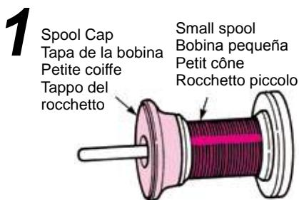
● Place a thread spool to spool pin and a spool cap onto the spool pin.
